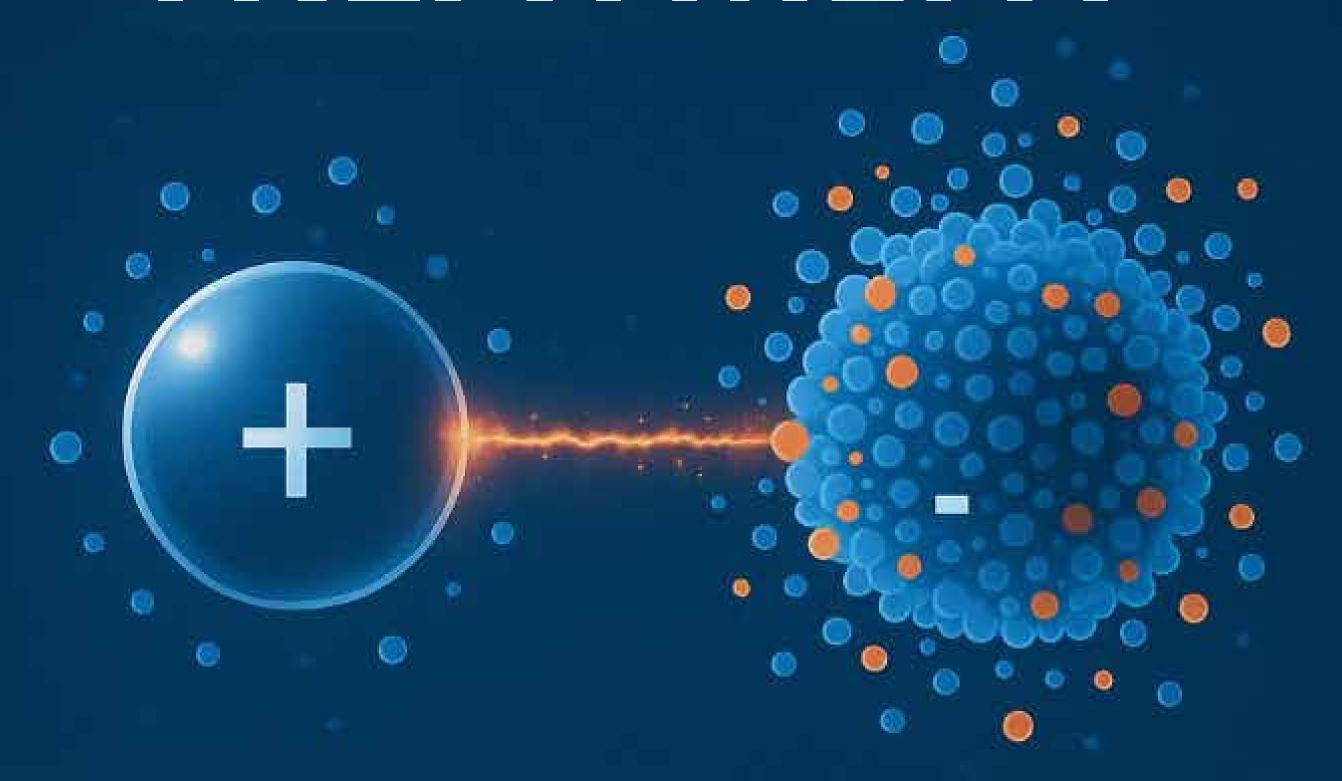
All ions in water are either positively charged or negatively charged. Impurities are attracted to the surface, making the floc bigger, which can then be easily filtered.
